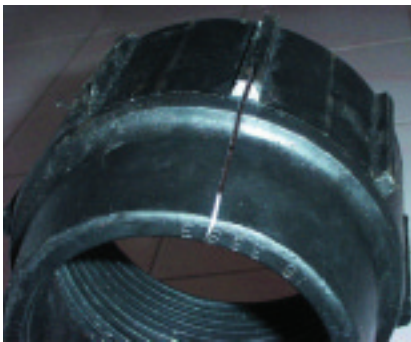
Failed nut with longitudinal split
