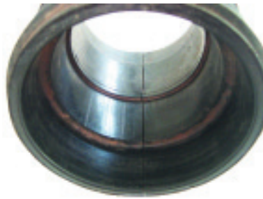
Failed body with longitudinal split
