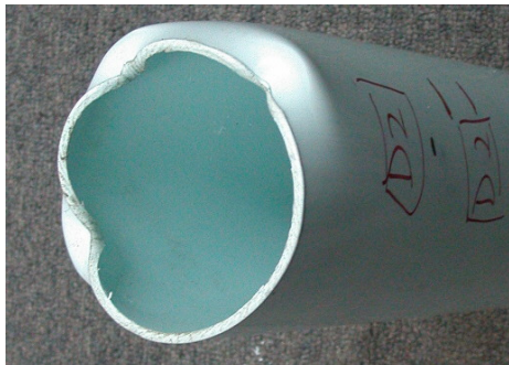
Fig 3: Spigot damage to PVC-O500 PN16 DN100 at 18 kN (1.8 tonnes eq) axial load
