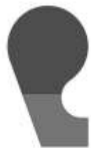
FIGURE 2 VXT ELASTOMERIC SEAL GASKET
