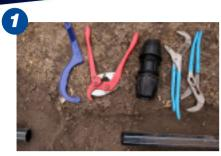
No special tools are required, standard multi-grips, pipe cutters or saw. If using a saw ensure there are no burrs.
