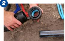
Remove the O-ring, then the split ring, collet and nut, then re-assemble the fitting and it is now ready to use.
