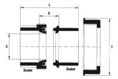
Note: This fitting is not intended to provide for angular misalignment. Do not overtighten.
