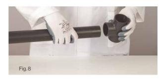
7) The pipe must be inserted in the fitting as soon and as quick as possible (after no more than 20-25 seconds is recommended).
