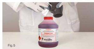
Leave the surfaces to dry for a few minutes before applying the Vinidex Type G Solvent Cement. Remember that, in addition to cleaning the joint surfaces, the Vinidex Priming Fluid also performs the important role of softening and preparing the surface to receive the solvent, an operation that enables a perfect joint to be obtained.
