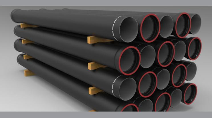
**LINX™** – Ductile iron pipes are supplied with 200g/m² zinc hot metal sprayed onto the external surface of the pipe plus 100micron bitumen finishing coat to inhibit corrosion.
