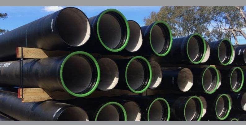
**LINX™** – Ductile iron pipes are supplied with 200g/m² zinc hot metal sprayed onto the external surface of the pipe plus 100micron bitumen finishing coat to inhibit corrosion.
