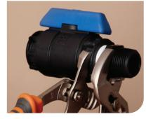
3. Using a pipe wrench or multigrips on the end caps only, further screw the blue handled ball valve into the male thread until tight. Where necessary ensure the male thread is held stationary to avoid it from moving. Do not use pipe wrench or multi-grips on the body of the blue handled ball valve.
