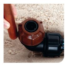
3. Cut copper pipe square. The fittings is pre-assembled and ready to use. Mark the depth of copper insertaion using 'pipe stop' marking or body flange as visual indicator. Remove any scale or burrs from the copper pipe.
