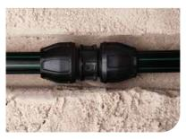
5. Position the insert in to the fitting and slide the nut up to engage the thread. The nut can now be tightened by hand and then a further 1/4 turn by wrench.
