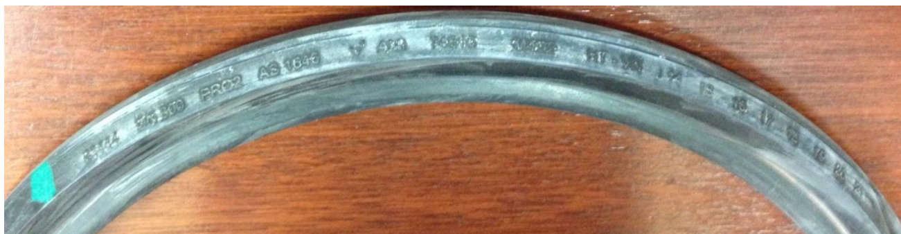
FIGURE 9: DN300 PRO2 HULTEC ELASTOMERIC SEAL MARKING
