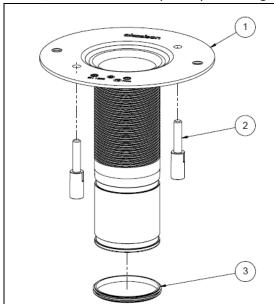
After the gutter outlet is installed the emergency overflow can easily be installed.
