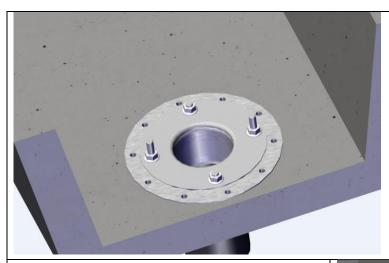
After the gutter outlet has been installed, a emergency overflow can easily be installed.
