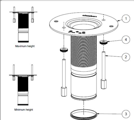
Variant 2 747592 emergency overflow element for 75mm gutter with 50mm elevation
